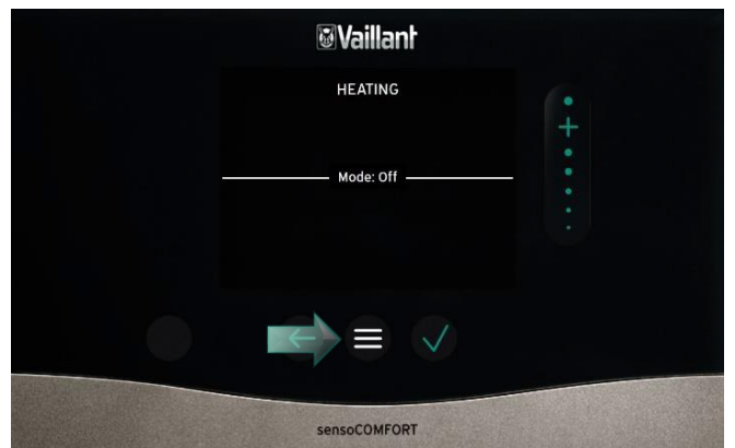
Heating now "Off" press menu to return
