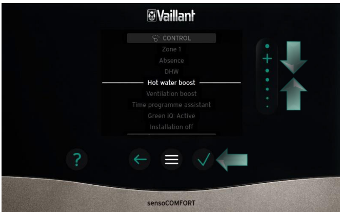
Scroll to "Hot water boost" and press Tick
